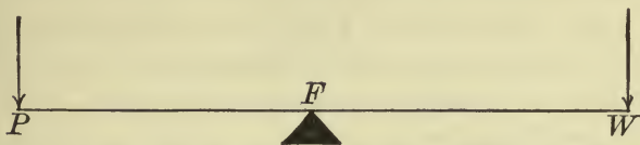
FIG. 40.—A lever of the first order. F , fulcrum; P , power; W , resistance or weight.
